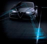
Lane Keep Assist alerts the driver if the vehicle is straying out if its lane and provides a corrective action to help automatically correct the vehicle's path and direct it back into the lane.
