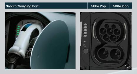
The new 500e is equipped with a CCS\* COMBO 2 Smart Charging Port that enables both public AC and DC charging as well as simple domestic AC charging. The port is positioned in the right rear side of the vehicle and gives immediate feedback on the charging status as well as possibility to manage set charging schedule or immediate charging.
